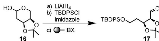
Scheme 4. Synthesis of key intermediate 17 . a) LiAlH 4 (1.4 equiv), THF, from 0 °C to 23 °C, 2 h, 95%; b) TBDPSCl (1.0 equiv), imid. (1.5 equiv), DMF, 23 °C, 2 h, 66%; c) PS-IBX (3.0 equiv), CH 2 Cl 2 , 23 °C, 2 h, 100%, DMF = dimethyl formamide, IBX = 2-iodoxybenzoic acid, TBDPS = tert -butyldiphenylsilyl.
